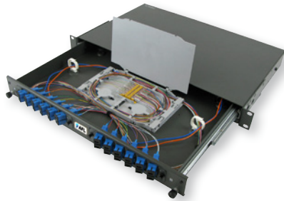
AFL FRE® 1RU Sliding Enclosure showing spliced SC 9 / 125 µm SM 2 m pigtails, 12 pk (P1SC2M-C12-900)
